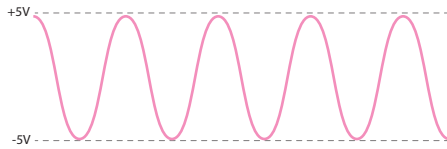
Figure 25: DPO VCO A Sine Wave: Base Frequency (No Control Voltage Applied)
